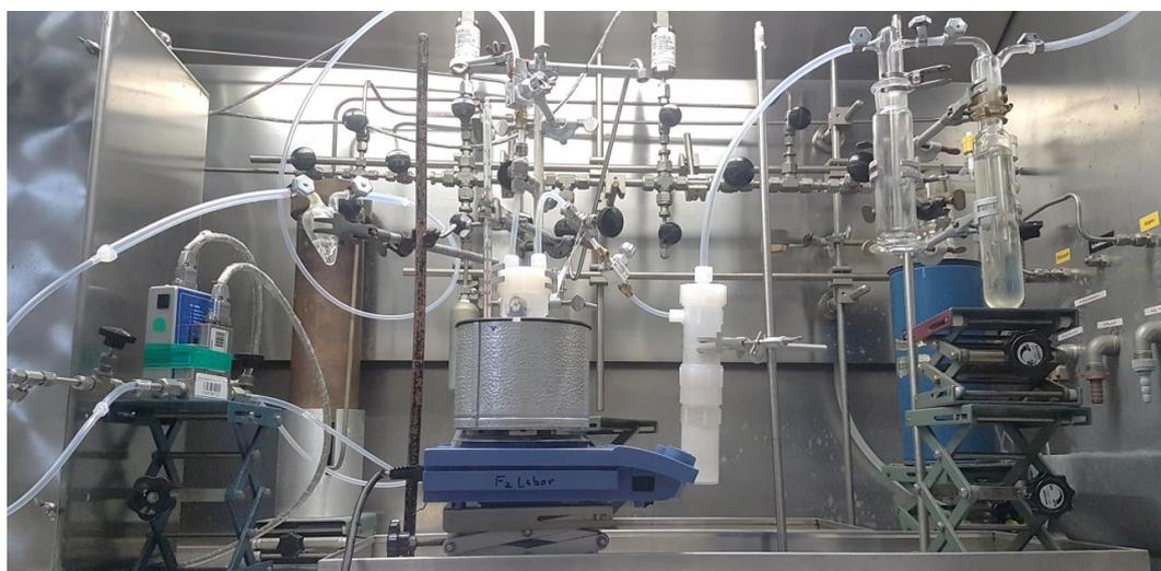
Figure 1: Monel Vacuum Line and Reaction Setup for Fluorinations in anhydrous HF.
